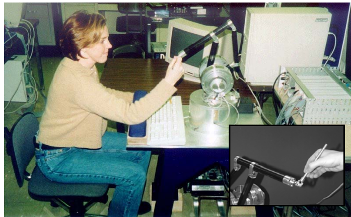
Figure 3-1. Human operator with the haptic interface (inset shows the human stylus grip).
